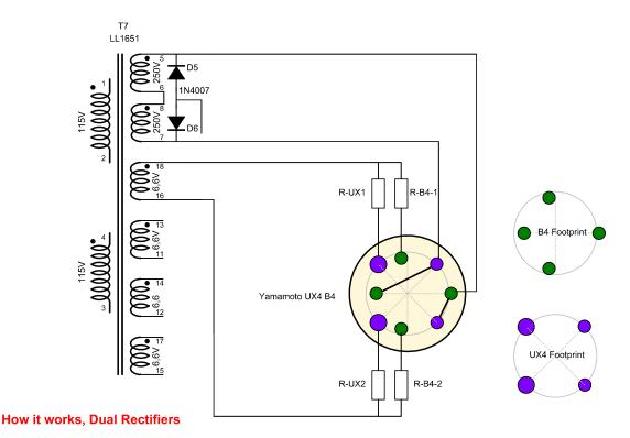
The Yamamoto Dual Socket UX4-B4 allows the use of American UX4 sockets and European B4 sockets together.
