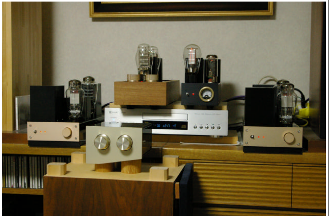
AV8B Single Line Amp With Tube based Voltage regulator 6000 Out AV8B : E_p=186V , I_p=15mA at E_g=18.2V
