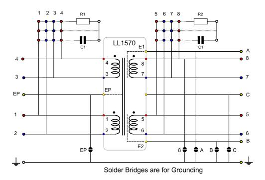
The Lundahl secondary designations for ground and shield, are here given for the LL1570, as an example, but can have different designations with other transformers. This is difficult and confusing.
