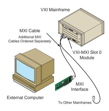
Figure 5. VXI System with MXI-Equipped Computer
