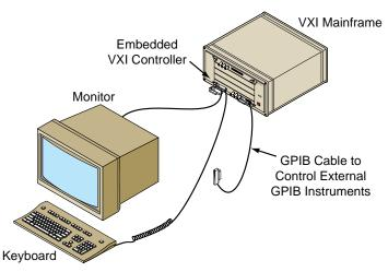
Figure 4. VXI System with Embedded Controller
