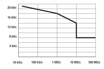
Figure 2. Flexible Resolution Sampling Rate vs Resolution
