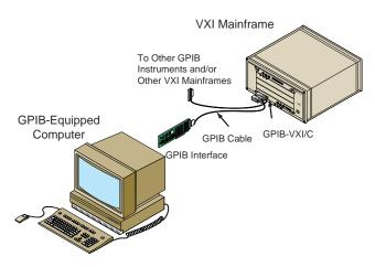
Figure 8. GPIB-Controlled VXI System
