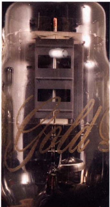
The massive plate structure of the NOS Genalex KT66 is a thing to behold.
