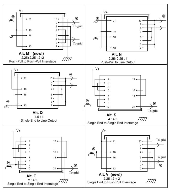
Alt.  $M^{\prime\prime}$  and Alt. V have been introduced to improve balance in PP applications
