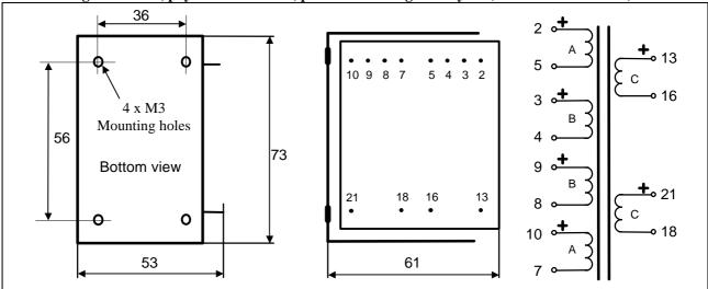
Max. current through any single section: 50~mA Isolation between primary and secondary windings / between windings and core: 4~kV / 2~kV
