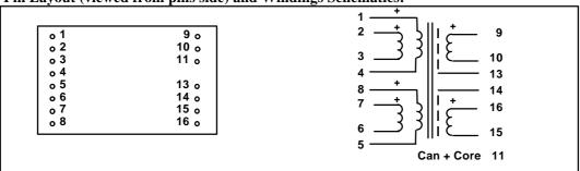
Spacing between pins: 2.54 mm (0.1")
