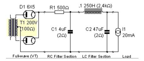
It is obvious, such a circuit must work as hum-free as possible. This means, a too large first capacitor would cause stray hum by too large current peaks throughout the whole circuit, and also from the tube itself. A too large second capacitor can cause saturation problems of the choke at start up, resulting in unwanted effects.
