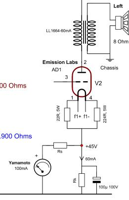
Minimum DC voltage over cathode resistor must be 1.6 Volt at full scale.
